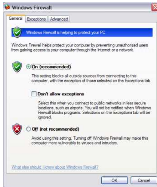
Figure 1.3: Windows Firewall settings, General tab.
